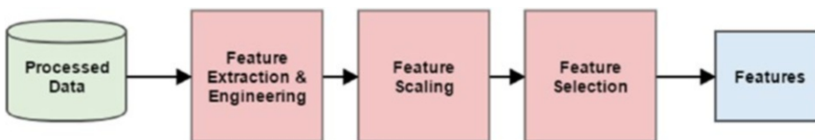
Figure 4-2. A standard pipeline for feature engineering, scaling, and selection
