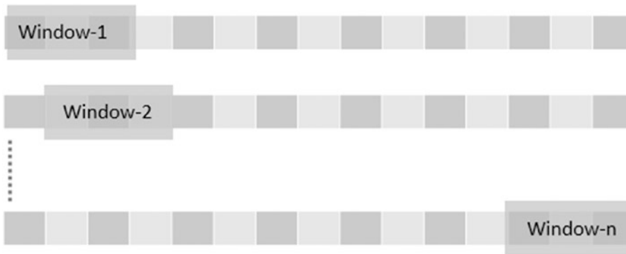
Figure 11-15. Rolling/sliding windows from original time series
